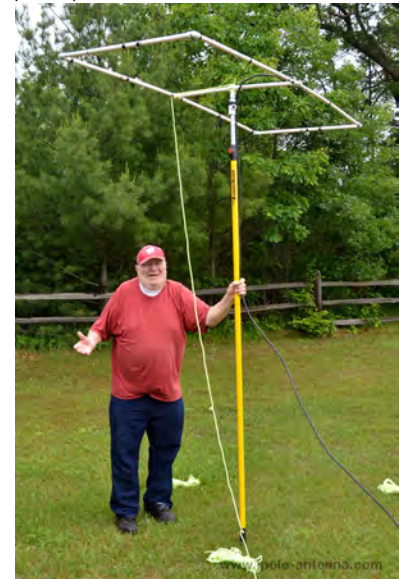
Figure 12: KB9VBR antennas: painter pole, pvc construction, 6m Moxon
