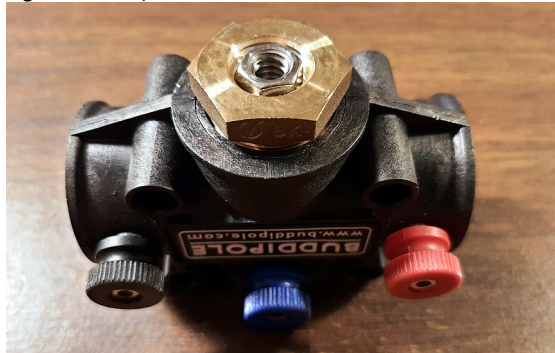
Figure 5: Adapter installed in Versatee
