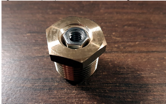
Figure 4: Coupler pressed home in bushing
