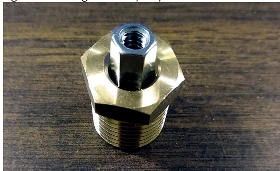
Figure 3: Bushing and coupler press-fit
